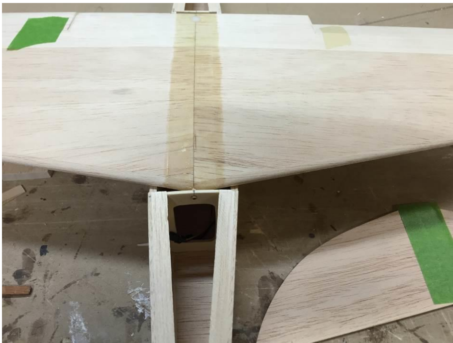
Drill out for wing hold down dowel at L.E. Fiberglass reinforce wing joint. Then glue in dowel.
